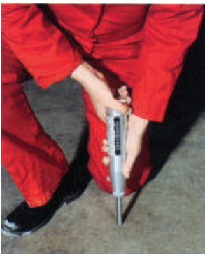
Schmidt hammer test
