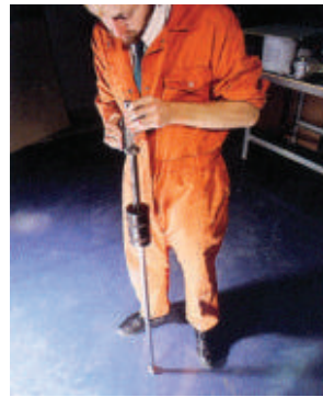
Impact resistance test
